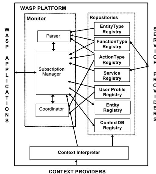
Figure 1. WASP architecture
