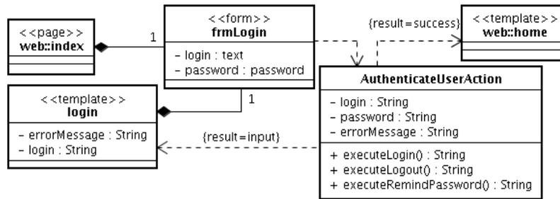
Figure 4. Navigation model for the Login scenario of Authenticate User use case (Portal LabES).
