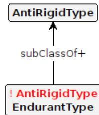
Fig. 11. Restrictive condition of a rigid or semi-rigid type specializing an anti-rigid one.
